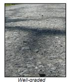
stones These mixtures are not suitable for drainage, but are preferred for use as surface aggregates as they tend to compact well to maintain desired road shape, lengthening grading cycles. This is also a key component in extending the road life cycle for traffic support.
