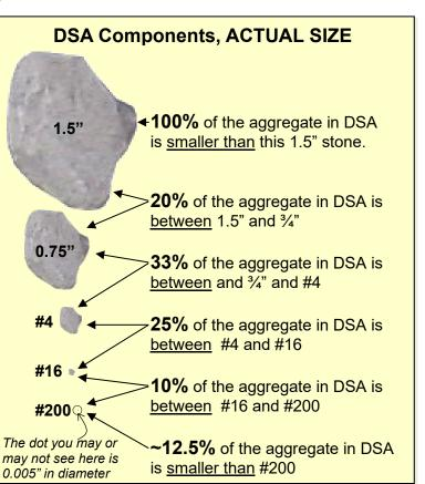
**Figure 1.** The specification is well graded from large pieces that give support, all the way down to the "fines", rock particles less than  $1/300^{\text{th}}$  of an inch. The illustration above shows the actual sizes of a "midline" or average DSA specification (roughly to scale when printed on 8.5" x 11" paper).
