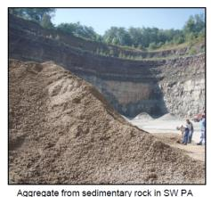
sedimentary rock such as limestone and sandstone. In the glaciated regions of NW and NE PA, aggregate is often mined glacial till, or pitrun gravel. In general, limestone is the hardest of the rocks, with shale being the softest, while pit-run varies widely in its usefulness as a road aggregate.
