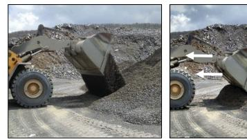
Figure 2. Laying out the sampling pile Figure 3. Forming the pad
