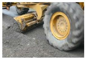
Figure 24: Wet material rolling off blade.
