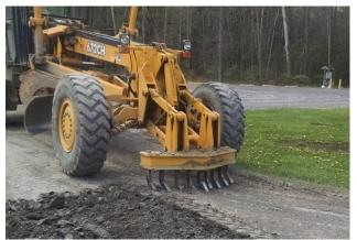
Figure 26. Grader equipped with scarifier teeth.
