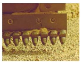
Figure 21. Individual carbide steel cutting bits
